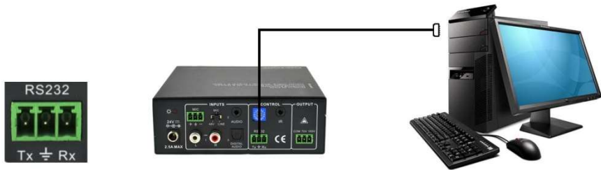
Figure 10 Connection of RS232 Port
