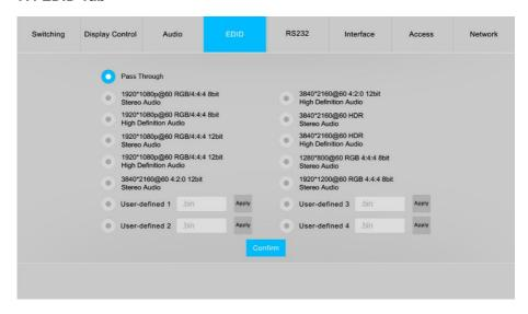
**Note:** Before select EDID in this tab, please ensure the 4-pin DIP switch on the rear panel is on the "1111" position.
