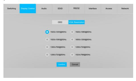
VGA output resolution can be selected as 1024x768@60Hz, 1280x720@50Hz, 1280x720@60Hz, 1360x768@60Hz, 1600x1200@60Hz, 1920x1080@50Hz, 1920x1080@60Hz (Default) or 1920x1200@60Hz.
