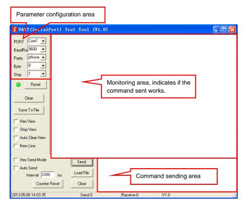
Please set the parameters of COM number, bound rate, data bit, stop bit and the parity bit correctly, then the RS232 commands can be sent in Command Sending Area.
